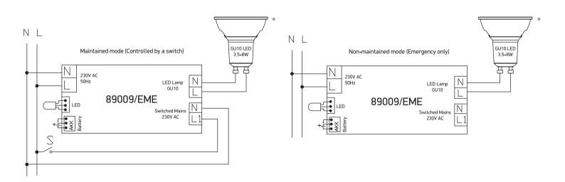
\* This kit will only operate with GU10 & E27 LED lamps suitable for 180V DC power supply. Most of the lamps in the market today are compatible however we recommend to test suitability before purchasing the lamps.
